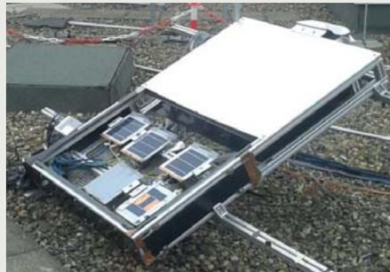
Fig. 1: Universal light-tight research installation (ULFI) for determining PID gradients.
